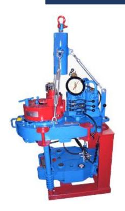
The FBU uses wrap around dies on the 04A05C unit and insert dies for the 04A09D unit. Dies come in a variety of configurations that include:
