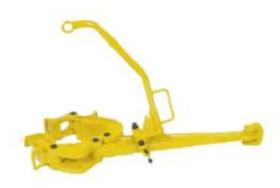
Type "LF" Tong is designed for water well drilling, seismographic, mining and geothermal rigs. Made from alloy steel, heat treated and magnetic partical inspected. Sizes range from 2 3/8" through 7 1/4" OD. An additional hinge jaw is available for pipe sizes from 7 1/4" to 8 5/8" OD. All steel specifications are certified.
