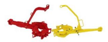
Type "DB" Tong covers drill pipe or casing sizes from 3 1/2" through 17" OD and like the "SDD" it has excellent durability, the tong is made from alloy steel, heat treated and magnetic particle inspected. All steel specifications are certified.
