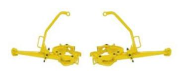
Type "H" Tong is ideal for light drilling and tubing work. Also used for seismographic, shot hole and exploration drilling. Like all other tongs a 3 Jaw design permits the jaws a uniform contact around the pipe. Jaw sizes range from 1.900" through 6 1/8" OD. All Steel specifications are certified.
