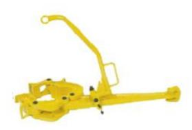
Type "B" Tong has established itself to be one of the best for toughness and durability and it is the most popular tong on the market, also can be ordered with an optional 36" lever. The tong is made from alloy steel, heat treated and magnetic particle inspected. Sizes range from 3 1/2" through 13 3/8" OD All steel specifications are certified.
