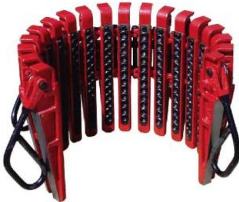
Casing Slips type "CMSXL" are designed to handle tubing or casing from 5 1/2" through 36" OD. These slips are light-weight, self-centering and made with a web type construction for support where it's needed. Slips are made from alloy steel, heat treated and tested for maximum durability. All steel specifications are certified.
