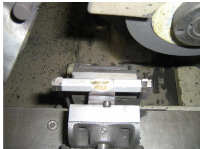
After this side is sharpened, the knife is stood on end & the cutting edge is placed level in the grinding machine.
