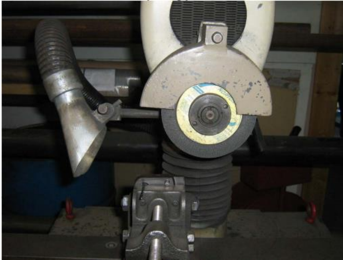
The set up in the grinding machine sharpens the top end of the long edge first.
